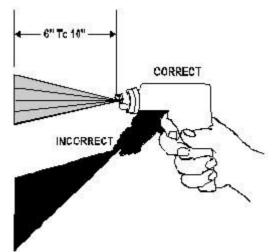
Hold the gun perpendicular to surface being sprayed
